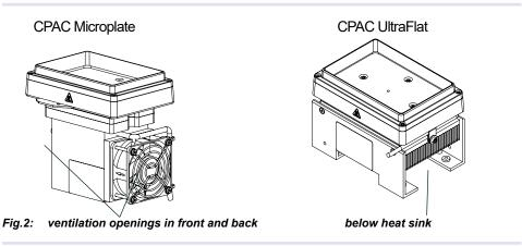
The CPAC Ultraflat is available in 2 types which differ in the direction of the ventilation.
