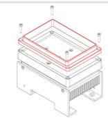
Fig.12: • Unscrew the 4 screws at the corner and remove mounting frame
