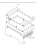
Fig.13: • Assemble the outer frame of flat bottom adapter with 2 screws
