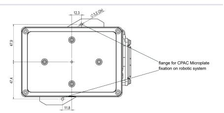
Fig.18: Drilling Scheme for CPAC Microplate
