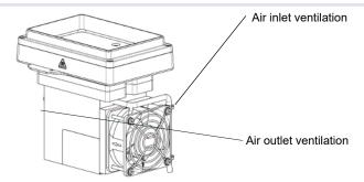
Fig.20: ventilation openings of CPAC Microplate
