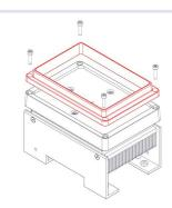
Fig.8: • Unscrew the 4 screws at the corner and remove mounting frame
