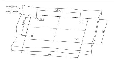
Fig.19: Drilling Scheme for CPAC Ultraflat
