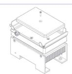
Fig.14: • Assemble the plate of flat bottom adapter with 1 screw in the middle
