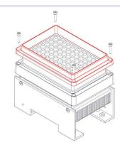
Fig.10: • Assemble PCR Adapter with mounting frame (to enclose the PCR Adapter) and 4 screws and tighten the four screws at the corner finger tight (respectively with 0,25Nm)
