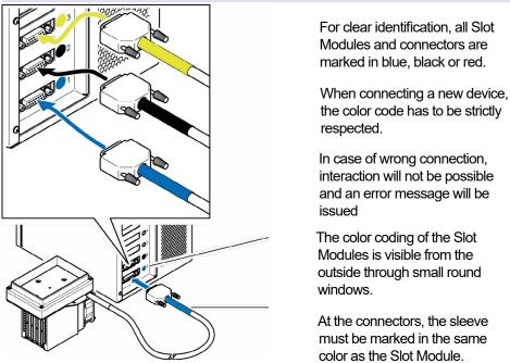
Fig.6: Connecting a heating/cooling/shaking device (image shows CPAC)
