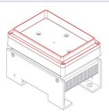
Fig.7: Mounting frame (red) screwed to CPAC device
