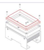
Fig.16: • Unscrew the 4 screws at the corner and remove mounting frame
