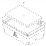
Fig.13: · Assemble the plate of flat bottom adapter with 1 screw in the middle
