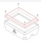
Fig.15: · Unscrew the 4 screws at the corner and remove mounting frame
