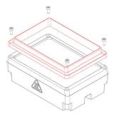
Fig.7: · Unscrew the 4 screws at the corner and remove mounting frame
