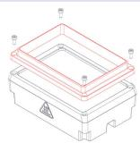
Fig.11: Unscrew the 4 screws at the corner and remove mounting frame
