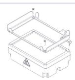
Fig.12: · Assemble the outer frame of flat bottom adapter with 2 screws
