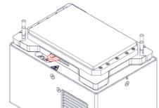
Fig.21: Clamp Mechanism "Closed"
