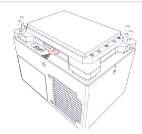
Fig.22: Clamp Mechanism "Open" with lever (in red)
