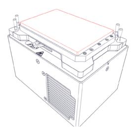
Fig.6: Heated area of Thermoshake AC (Teleshake 95 AC is similar)
