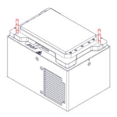
Fig.5: Fixation Pins of Clamp Mechanism
