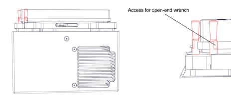
Fig.15: Removal of Fixation Pins
