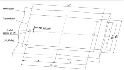
Fig.18: Drilling Scheme
