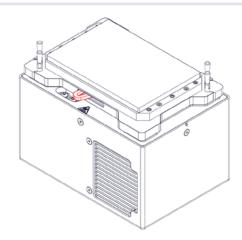
Fig.4: Clamp Mechanism "Closed"
