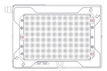
Fig.17: Device with installed PCR adapter plate (3 screw holes used )
