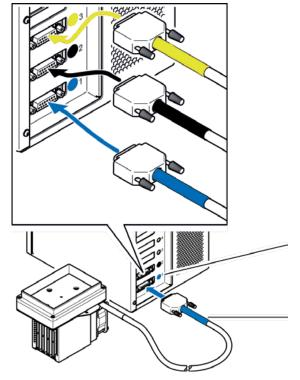
For clear identification, all Slot Modules and connectors are marked in blue, black or yellow.
