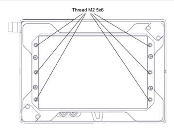
Fig.16: Threaded holes to fix or unfix the adapter plates
