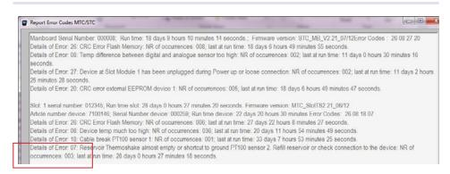
Fig.26: Example: Details of Error 07: no. of occurrences: 003, in case of an increase in 2nd report to 004 → refill is required
