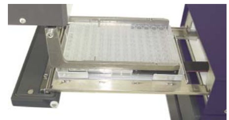
7300003 Incubator MP gripper access, similar to Incubator Shaker
