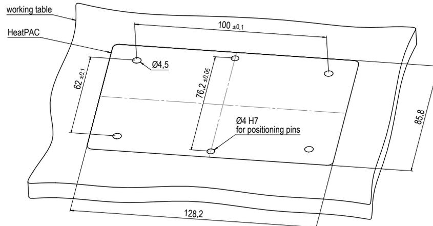
**Fig.18: Drilling Scheme**
