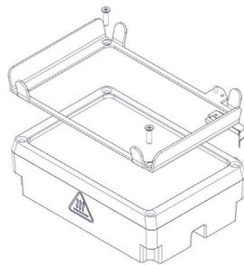
**Fig.12:** · Assemble the outer frame of flat bottom adapter with 2 screws
