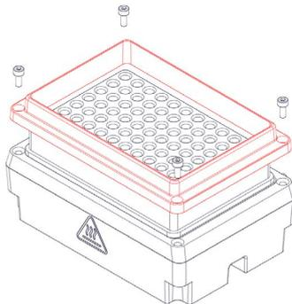
**Fig.9:** · Assemble PCR Adapter with mounting frame (to enclose the PCR Adapter) and 4 screws and tighten the four screws at the corner finger tight (respectively with 0,25Nm)
