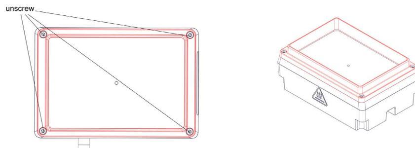
**Fig.6: Mounting frame (red) screwed to HeatPAC device**
