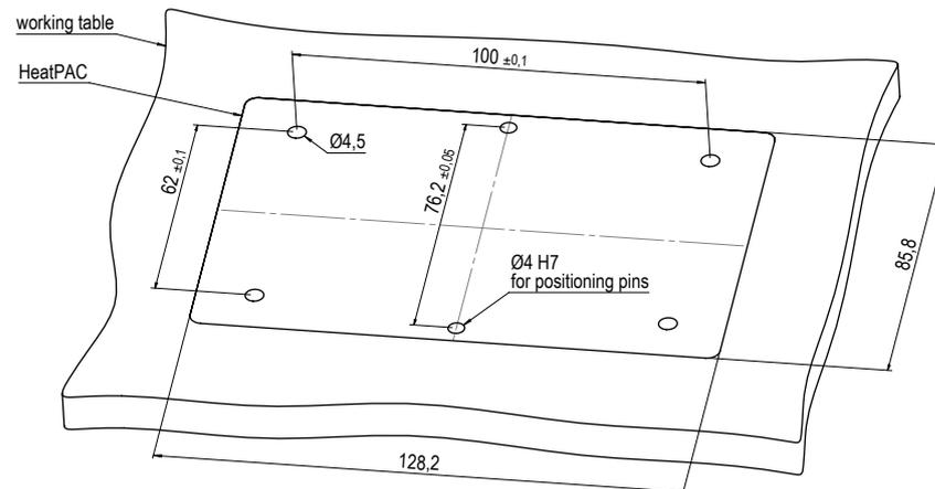
**Fig.18: Drilling Scheme**
