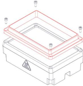
**Fig.15:** · Unscrew the 4 screws at the corner and remove mounting frame
