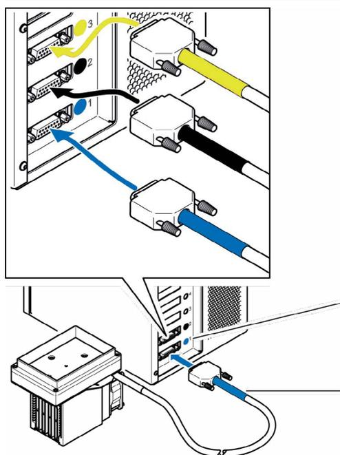
For clear identification, all Slot Modules and connectors are marked in blue, black or red.
