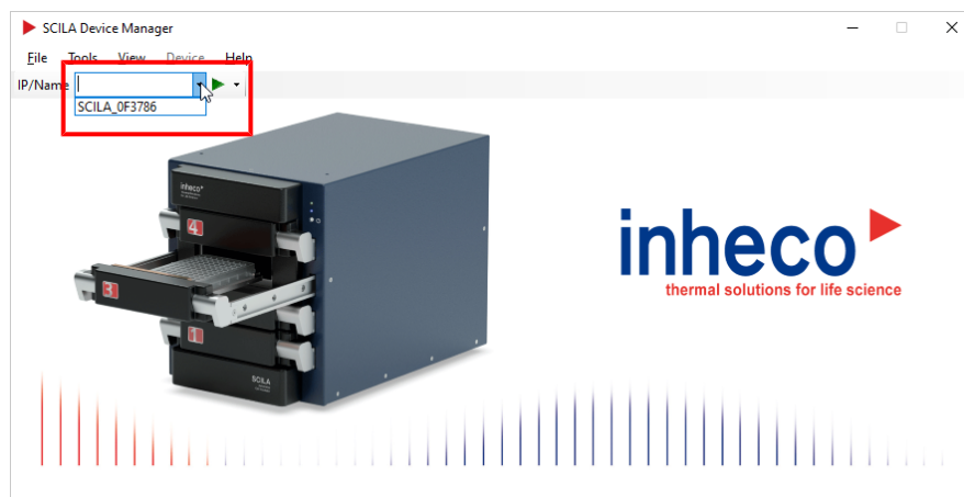
Illustration 7: IP/Name window drop-down menu for selecting an SCILA with its node name
