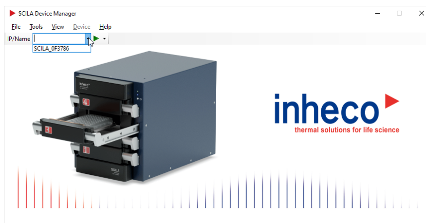
Illustration 5: IP/Name window drop-down menu for selecting an SCILA with its node name
