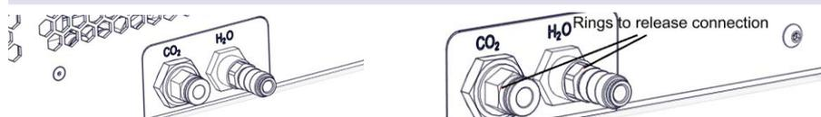
Fig.7: CO<sub>2</sub> and H<sub>2</sub>O quick connector at the back of the SCILA
