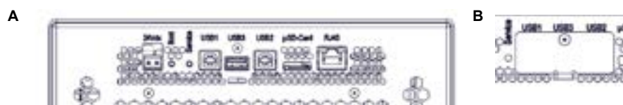
Fig.6: SCILA connectors at the back (A) access to all connectors, but the covered USB connectors are covered (B) as they are for INHECO use only
