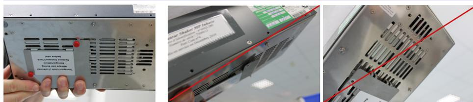
Fig.26: correct installed transportation lock and **incorrect** installed transportation lock
