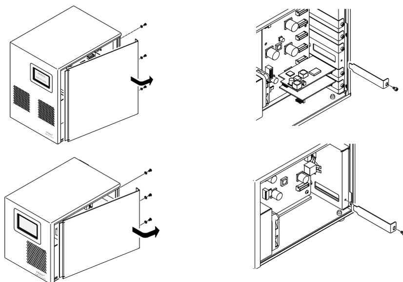
**Fig.7: Removing cover plate (MTC shown at top and STC shown below)**
