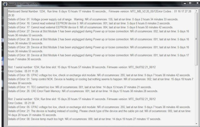
In the first line the information about the overall run time of mainboard, the firmware version of mainboard and the error codes are displayed.
