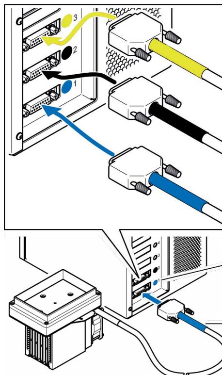
For clear identification, all Slot Modules and connectors are marked in blue, black or yellow.
