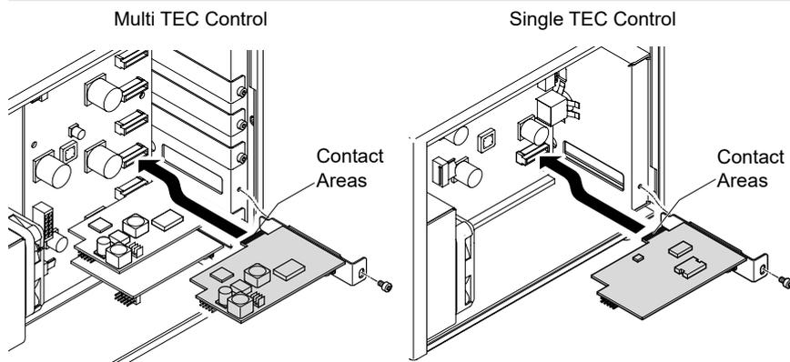
**Fig.8: Insert Slot Module**
