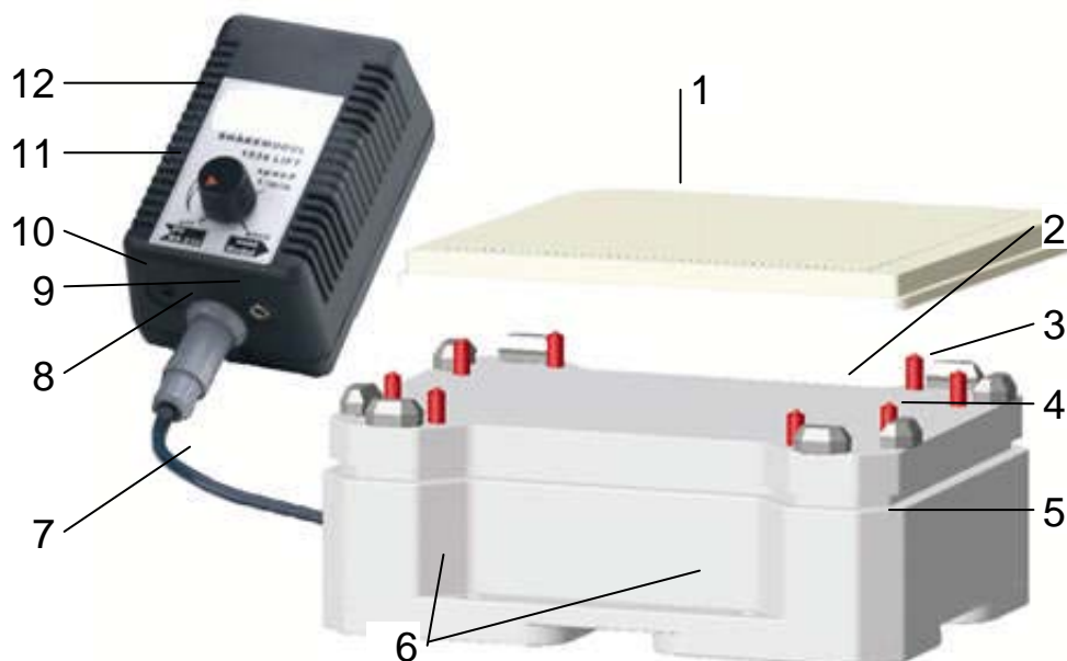
Figure 3: Magnetic shaker TELESHAKE 1536 LIFT with the control unit SHAKEMODUL 1536 LIFT
