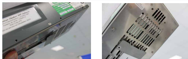
Fig.4: incorrect installed transportation lock
