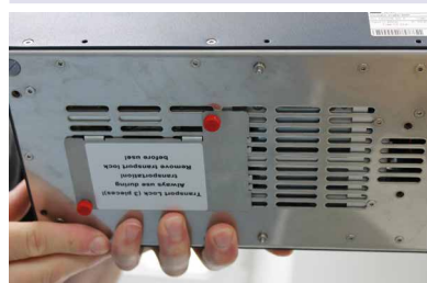
Fig.3: correct installed transportation lock
